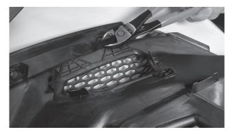
Step 10 - Using side cutters or a razor knife, remove the four (4) mounting tabs on the bottom side of the panel around the speaker opening to provide proper clearance for the pod installation. **Note:** These D0 NOT need to be perfectly flush with the back of the panel.
