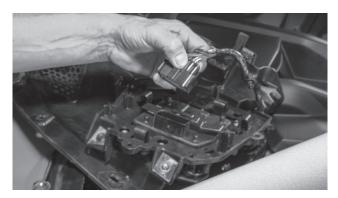
Step 6 - On the passenger side, locate and remove five (5) T-30 Torx screws, one with 10mm nut, and two (2) pushpin rivets from the passenger's side upper dash panel.
