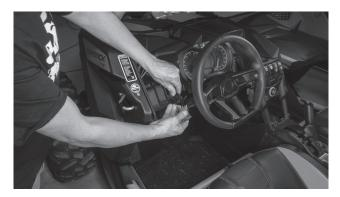
Step 3 - Release and push the steering wheel to its lowest position for proper clearance.
