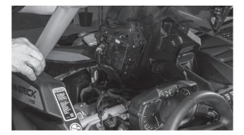
Step 5 - Once the panel is loose, disconnect the computer harness from the computer module attached to the panel and remove the panel from the vehicle. **Note:** It is not necessary to remove the computer module from the panel for installation of the speaker pod.
