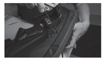
Step 16 - Once started, install the coarse thread screw through the single bottom hole into the pod and tighten.
