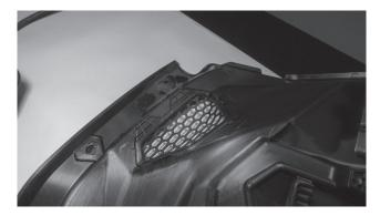
Step 11 - Turn the panel over and locate the three (3) dimples around the molded speaker grill. Two (2) on top and one (1) on bottom of the grill area.
