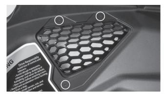
Step 12 - Using a <sup>3</sup>/<sub>16</sub>" drill bit, drill though the panel at each dimple location.
