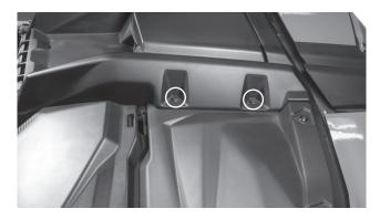
Step 7 - With hardware removed, lift up on the dash panel releasing the harness clips from the bottom side as you do.
