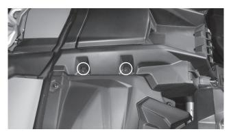
Step 2 - Disconnect the light switch harness from the back of the switch. **Note:** If any additional switches are mounted in this panel, disconnect at this time. If necessary, label harnesses to ensure proper reconnection.
