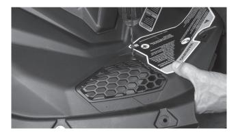
Step 13 - On the speaker pods, locate the single molded dimple at the bottom of the pod face.
