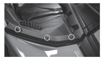
• Two (2) pushpins located on left side of the panel at top center tray.
