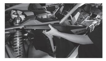
Step 5 - The driver's inner footwell panel will also be free now, remove it and set it aside for the installation process.
