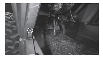
• One (1) located in the front corner by the headlight with a 10mm nut.
