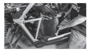
Step 6 - On the passenger side, remove the gas cap cover panel and set aside.
