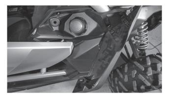
Step 7 - Locate and remove twelve (12) screws using a T30 Torx driver and 10mm wrench where needed.
