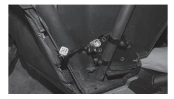
Step 22 - Holding the pod in place against the inside panel, align the threaded inserts with the holes in the mounting plate.
