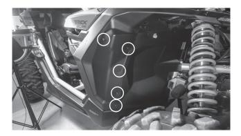
One (1) located at the top of the fender forward of the roll cage behind cover. Note: This is a longer bolt than the rest being removed.
