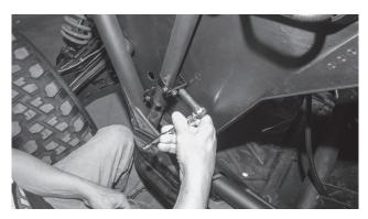
Step 21 - Pass the driver side pod's harness through the forward most hole.
