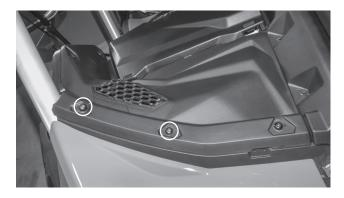
Step 8 - Remove two (2) metal clips and plastic retaining plates from the underside of the fender section attaching it to the passenger side hood trim piece.
