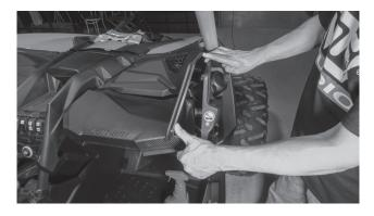
Step 10 - Loosen the topmost hose clamp securing the fender assembly to the filler tube and slide the clamp down out of the way.
