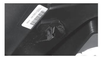
Step 4 - Once the clips are removed, lift up on the hood trim and lift the outer fender piece up and back toward the rear of the vehicle to disengage it. Set it aside.
