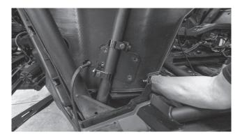
Step 23 - Install four (4) 10mm bolts through the plate and secure the pod in place.
