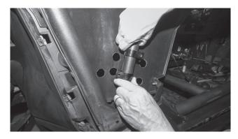
Step 18 - Using two (2) longer 10mm bolts supplied, install the two saddle pieces into the hoop clamps leaving them loose enough to move up and down the frame tube.
