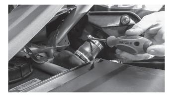
Step 11 - Lift up on the hood trim piece and pull the fender up and away from the vehicle to remove it. Once removed, set aside. **Note**: Once removed, cover or stuff a clean rag into the filler tube to prevent gas fumes from escaping.
