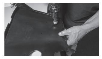
Step 15 - Once the holes are drilled, temporarily reinstall the interior panel by reinserting the screw removed from the lower door jamb location.
