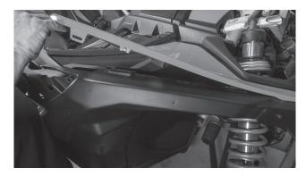
Step 12 - Starting with the removed driver's interior panel, locate and align the driver side template supplied with the speakers as shown. **Note**: Templates and mounting plates are marked relative to the side of the vehicle they are for. Ensure you pay attention to and use the appropriate parts for installation for proper fitment.
