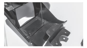
Step 6 - Sliding the plate toward the rear of the kit, install the radio into the kit opening from the rear making sure the top of the radio is between the kit face and compression plate. Once in position, press the radio forward into the opening until it is flush with the front and aligned with the pre-molded screw holes.
