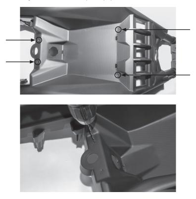
Step 3 - Using a 1" hole saw, drill a hole in the top of the dash to pass the wiring harness through. Our recommended location is indicated in the picture. **Note:** The 12-volt power port can be removed and used to pass the harness through the dash if you do not desire to drill a separate hole. This will require the removal of the center dash console panel to remove the power port.
