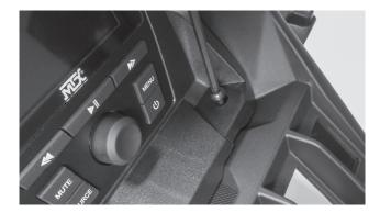
Step 12 - With the radio secure, make the appropriate electrical connections to complete the install such as power, ground and remote turn on for amplifiers.
