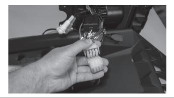
Step 11 - With connections made, collect the wire harness under the kit shroud and place the radio kit on top of the dash aligning it with the four (4) holes drilled earlier. Making sure all wires are tucked under the kit, secure it in place with the four (4) screws provided
