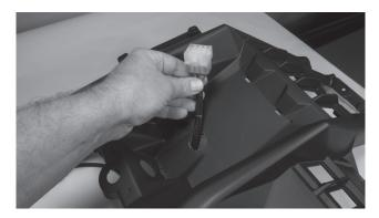
Step 10 - At this time, any RCA signal wires should be fed up through the hole for connection to the radio unit. Once wires are in place, make the appropriate connections to the radio.
