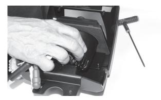
Step 7 - Using the two (2) longer screws, secure the bottom of the radio to the kit.
