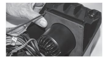
Step 8 - While pressing the pressure plate forward against the radio chassis, tighten the two (2) screws left loose in Step 5.
