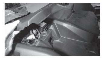
Step 2 - Locate the four (4) dimples formed into the tray area on the top center dash. Two are located toward the front and two are at the rear under the cover that was just removed. Using a  $\frac{1}{2}$  drill bit, drill through the dimples just enough to expose the existing boss located below. **Caution**: Drilling deeper can damage the bosses beneath and prevent proper installation of the dash kit.
