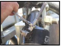
2.5 For integral or remote reservoir *(not piggyback)* struts, order PA-235-D adapter kit to provide needed clearance between T-fitting and compression damping knob. The vent
